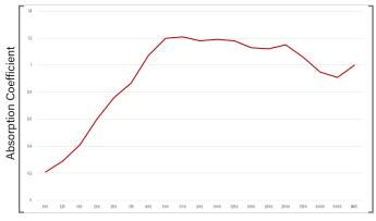
Sound can either be absorbed, reflected or diffused. In many rooms, flat reflective surfaces can cause interfering reflections and excessive reverberation, which corrupts music quality, speech clarity and general hearing comfort. One approach to controlling these reflections and excess reverberation time is to use absorptive panels. RPG have developed a simple and cheap method of fixing these panels which allows easy mounting and demounting of Absorbor™ panels.
