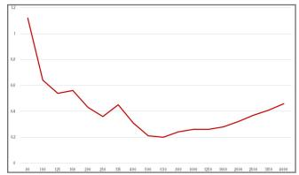
The Modex Corners are low frequency membrane sound absorbers designed to fine tune the modal distribution in a small room such as a studio control or music listening room. Designed to sit into a corner, the tuning frequencies available for Modex Corners are 40, 63 and 80Hz. The units are designed to cover approximately 1/3 octave above and below the tuning frequency.
