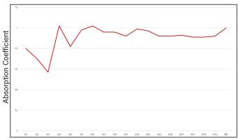
The High Impact Absorber™ Panel consists of a multi-density, high performance acoustical core with hardened square or shaped edges and wrapped in an acoustical fabric. The High Impact Absorber ™ Panel offers durability and tackability with little deviation in the performance bandwidth between 100Hz and 5000Hz, yielding a balanced NRC up to 1.00.
