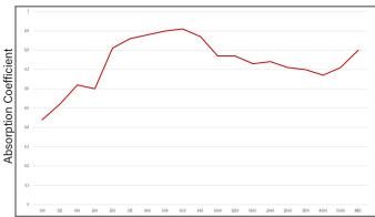
The Expo panel system is the ultimate synergy between acoustical technology and architectural panel design. Utilizing an optimal binary pattern of perforations through a recycled, Class A fire rated, ULEF and FSC certified wood panel, the Expo achieves an excellent balance of sound absorption across the NRC frequency bands while preserving the ambiance of the space with high frequency diffusion.
